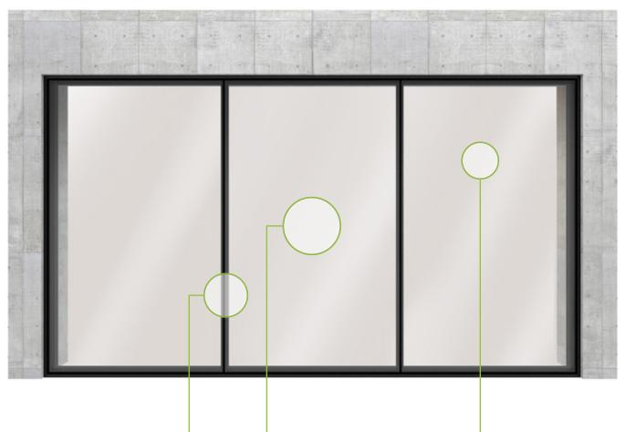
Slimline look Flush-fitted all-glass look on the external façade with slimline joints Schüco Façade FWS 50 SG.SI Harmonious all-glass façade look with flush-fitted glazing without visible mechanical fixings
