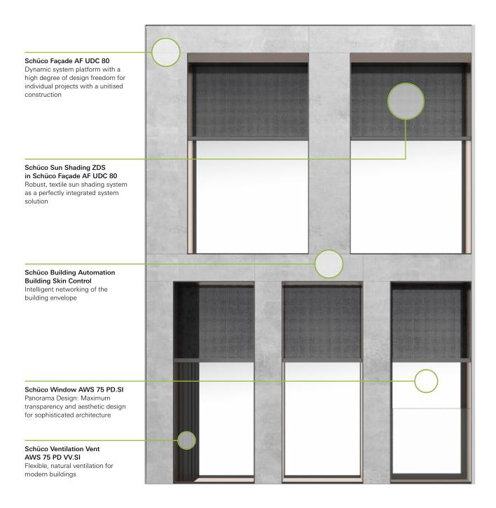
Schüco unitised façade with integrated sliding door, ventilation system with ventilation function and sound-absorbing façade units (concept)
